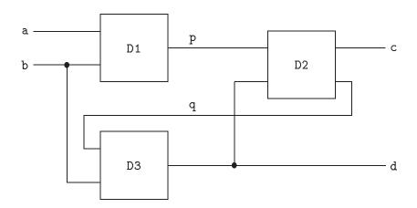
This device is built by connecting together three component devices D1, D2 and D3. The external lines of D are a, b, c and d. The lines p and q are internal and are not connected to the 'outside world'. (External lines might correspond to the pins of an integrated circuit, and internal lines to tracks.)
