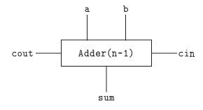
The lines cin and cout carry 1-bit words and the lines a, b and sum carry n-bit words. We will model 1-bit words as booleans and n-bit words as functions from natural numbers to booleans. Thus the 4-bit word 1101 is represented by a function f such that f(0)=T, f(1)=F, f(2)=T and f(3)=T. To relate words to numbers we use a function Val such that Val(n, f) is the number denoted by the (n+1)-bit word  $f(n)f(n-1)\cdots f(0)$ . Val can be defined by primitive recursion.
