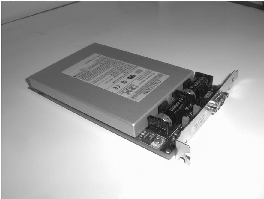
**Figure 16.1:** The IBM 4758 cryptoprocessor (courtesy of Steve Weingart)
