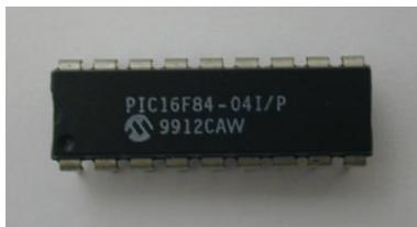
Figure 3. Microcontroller PIC16F84
