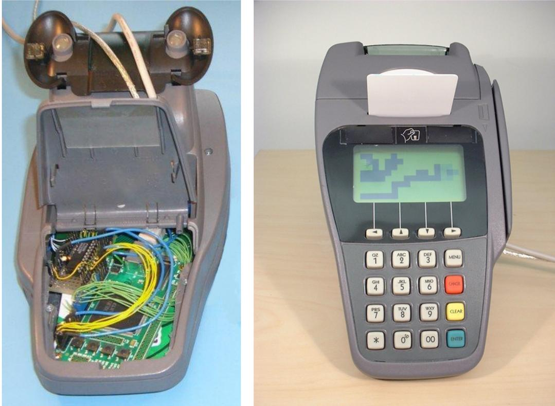
Figure 8: Modified Chip and PIN terminal, playing Tetris
