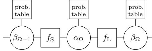
**Figure 6:** The factor graph for round  $\Omega$  of the ASCON permutation. State variables  $\beta_{\Omega-1}$ ,  $\alpha_{\Omega}$ , and  $\beta_{\Omega}$  shown here each represent 320 single-bit variable nodes, respectively.
