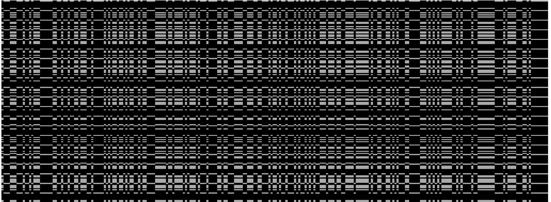
The text “Tempest in a Teapot” encoded in ASCII (padded with start- and end-of-text control characters) DSSS-modulated.
