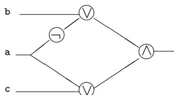
is a Boolean circuit representing the Boolean proposition  $(\neg a \vee b) \wedge (a \vee c)$ ; giving particular high (**T**) or low (**F**) voltages to the input wires **a**, **b**, **c** on the left, determines, as we move from left to right, a particular value of high (**T**) or low (**F**) on the output wire, at the extreme right.
