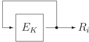
Again, the key  $K$  should be replaced before in the order of  $2^{\frac{n}{2}}$   $n$ -bit blocks have been generated, otherwise the random block generator is likely to enter a cycle where  $R_i = R_{i-k}$  for some  $k$  in the order of  $2^{\frac{n}{2}}$ .
