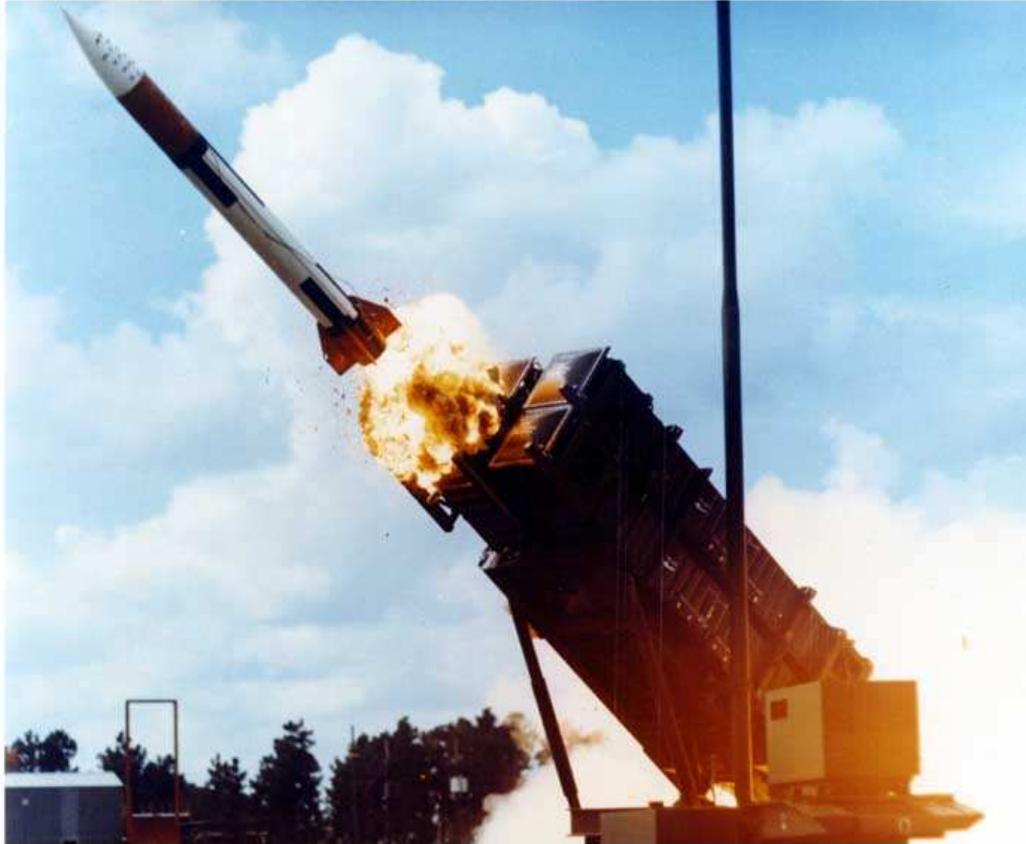
Patriot missile interceptor fails to intercept due to 0.2 second being the 'recurring decimal'  $0.0011001100\dots_2$  in binary (1991).
