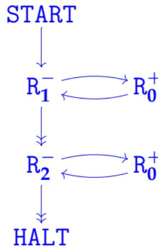
**Claim:** starting from initial configuration  $(0, 0, x, y)$ , this machine's computation halts with configuration  $(4, x + y, 0, 0)$ .
