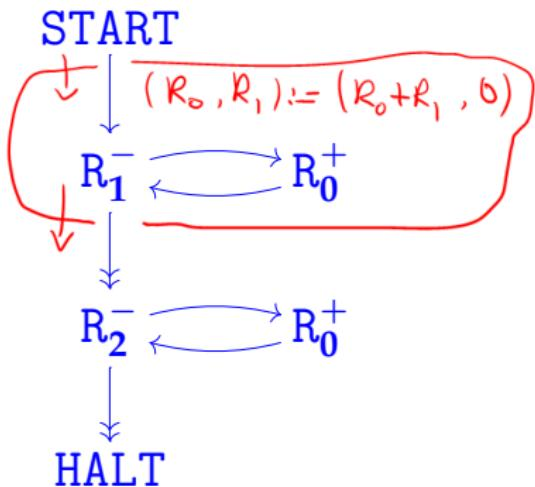
**Claim:** starting from initial configuration  $(0, 0, x, y)$ , this machine's computation halts with configuration  $(4, x + y, 0, 0)$ .
