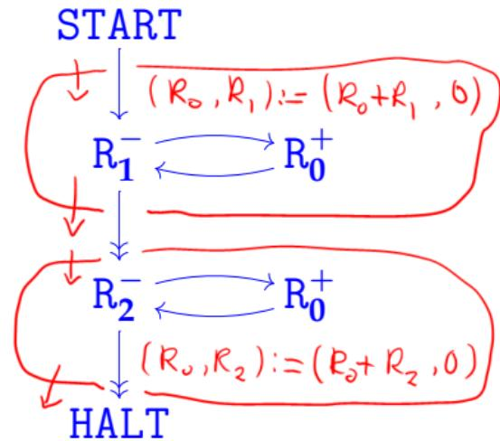
**Claim:** starting from initial configuration  $(0, 0, x, y)$ , this machine's computation halts with configuration  $(4, x + y, 0, 0)$ .
