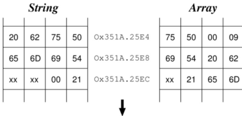
Both ASCII and Unicode are represented in memory as either strings or arrays: e.g. "Pub Time!" ( $0x50 = 'P'$ ,  $0x75 = 'u'$ , etc)
