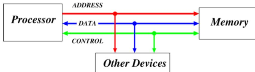
Collection of shared communication wires: low cost, versatile but potential bottleneck. Typically comprises **address lines** (determine how many devices on bus), **data lines** (determine how many bits transferred at once) and **control lines**,
