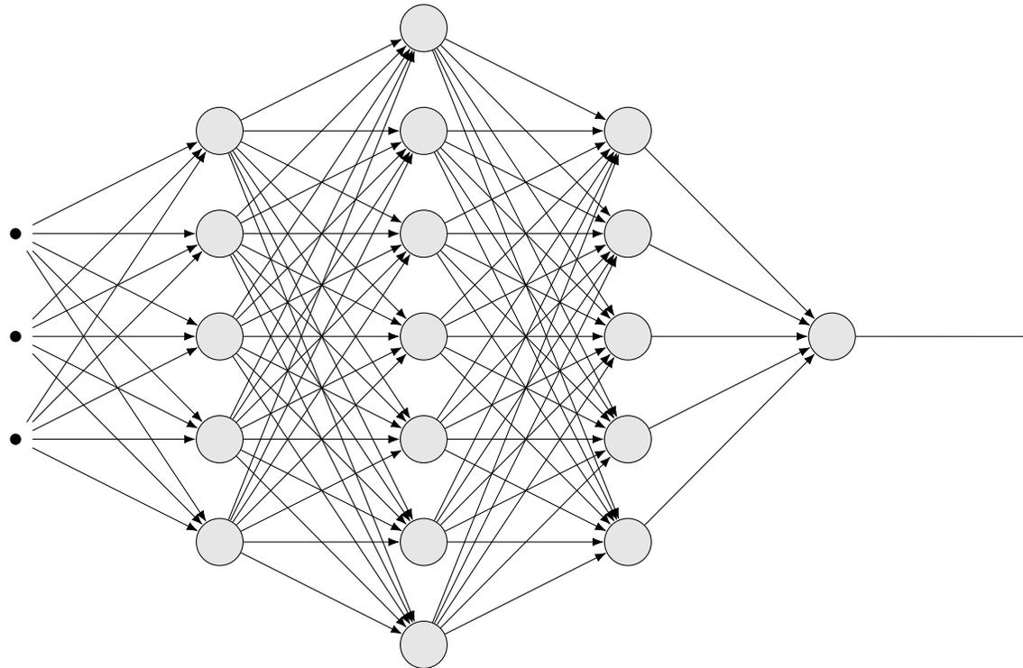
Here, each *node* is a perceptron and each *edge* has a weight attached.
