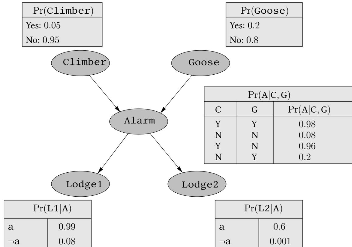
$$\Pr(C, G, A, L1, L2) = \Pr(C) \Pr(G) \Pr(A|C, G) \Pr(L1|A) \Pr(L2|A).$$
