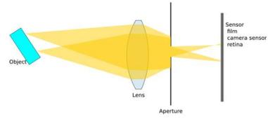
Aperture (introduced behind the lens) reduces the amount of light reaching sensor, but it also reduces blurriness from defocus (increases depth-of-field).
