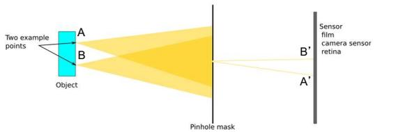
Pinhole masks all but only tiny beams of light. The light from different points is separated and the image is formed.
