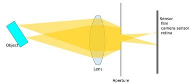
Aperture (introduced behind the lens) reduces the amount of light reaching sensor, but it also reduces blurriness from defocus (increases depth-of-field).
