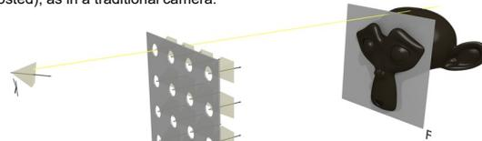
If we have a proxy geometry, we can project on that geometry instead – the rendered image will be less ghosted/blurry
