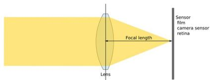
Focal length – length between the sensor and the lens that is needed to focus light coming from an infinite distance.
