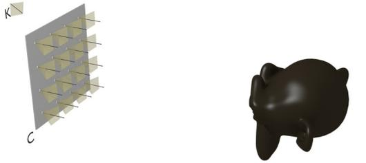
We want to render a scene (Blender monkey) as seen by camera K. We have a light field captured by a camera array. Each camera in the array has its aperture on plane C.
