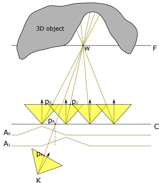
Figure 1: Light field rendering for the novel view represented by camera  $K$ . The pixels  $P_K$  in the rendered image is the weighted average of the pixels values  $p_1, \dots, p_N$  from the images captured by the camera array.
