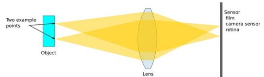
Lens can focus a beam of light on a sensor (focal plane).
