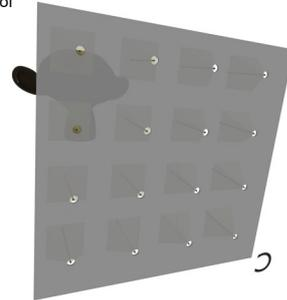
Each camera in the array provides accurate light measurements only for the rays originating from its pinhole aperture.
