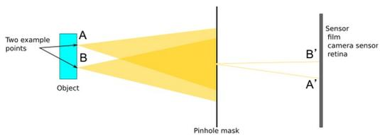
Pinhole masks all but only tiny beams of light. The light from different points is separated and the image is formed.
