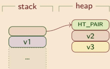
Place pointers to heap on stack
