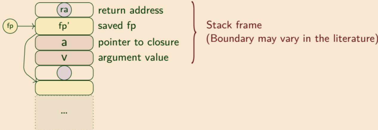
Executing code for closure at heap address a after it was applied to argument v.
