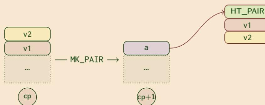
The pair is freshly allocated on the heap
