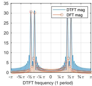
Applying the discrete Fourier transform (DFT) to an  $n$ -element long real-valued sequence samples the DTFT of that sequence at  $n/2 + 1$  discrete frequencies.
