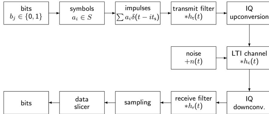
IQ up/down conversion: only required for pass-band channels (e.g., radio)
