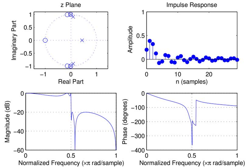
order: 5, cutoff frequency:  $0.5 \times f_s/2$ , pass-band ripple: -3 dB, stop-band ripple: -20 dB
