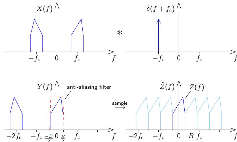
Shifting the center frequency  $f_c$  of the interval of interest to 0 Hz (DC) makes the spectrum asymmetric. This leads to a complex-valued time-domain representation
