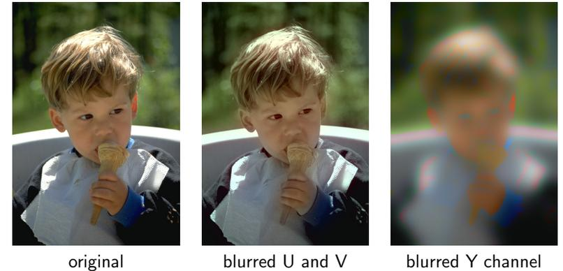
In the centre image, the chrominance channels have been severely low-pass filtered (Gaussian impulse response
