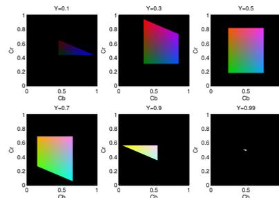
Modern image compression techniques operate on  $Y$ ,  $Cr$ ,  $Cb$  channels separately, using half the resolution of  $Y$  for storing  $Cr$ ,  $Cb$ .
