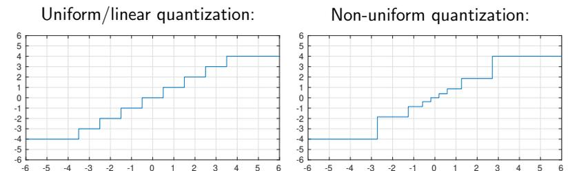
Quantization is the mapping from a continuous or large set of values (e.g., analog voltage, floating-point number) to a smaller set of (typically  $2^8$ ,  $2^{12}$  or  $2^{16}$ ) values.
