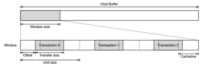
Figure 3: Host buffer layout and access parameters
