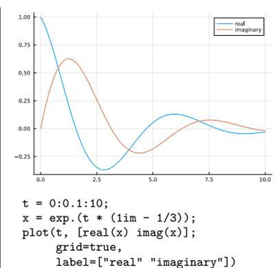
Function plot expects a vectors of  $x$  coordinates, and a vector or matrix of  $y$  coordinates, one column per curve. Use plot! to add additional curves with independent  $x$  coordinates.
