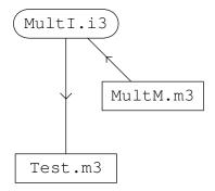
In this representation, a box with rounded ends represents an interface and a rectangular box represents a module. The arrows represent the directions of imports and exports. Augment this diagram to include the file containing the interface Main and any other interfaces and modules used directly or indirectly by the interface and module you have written. [7 marks]
