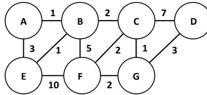
(a) In the above network, use Dijkstra’s shortest-path algorithm to compute the shortest path from E to all network nodes. Show your working in a table: each column indicating a destination node, each row indicating an iteration of the algorithm. [10 marks]
