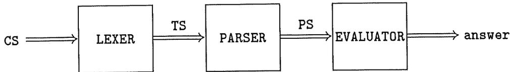
Figure 1.3: A pipelined evaluator for arithmetic expressions
