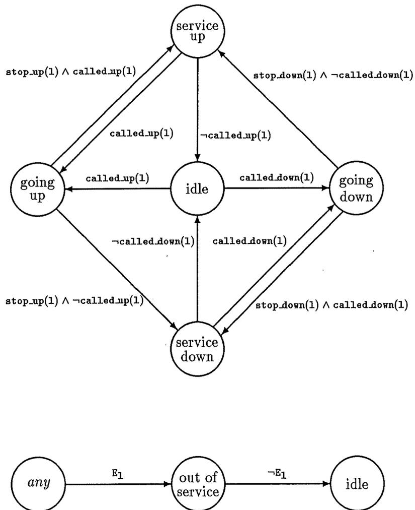
Figure 9.4: A state transition diagram for the lift system.
