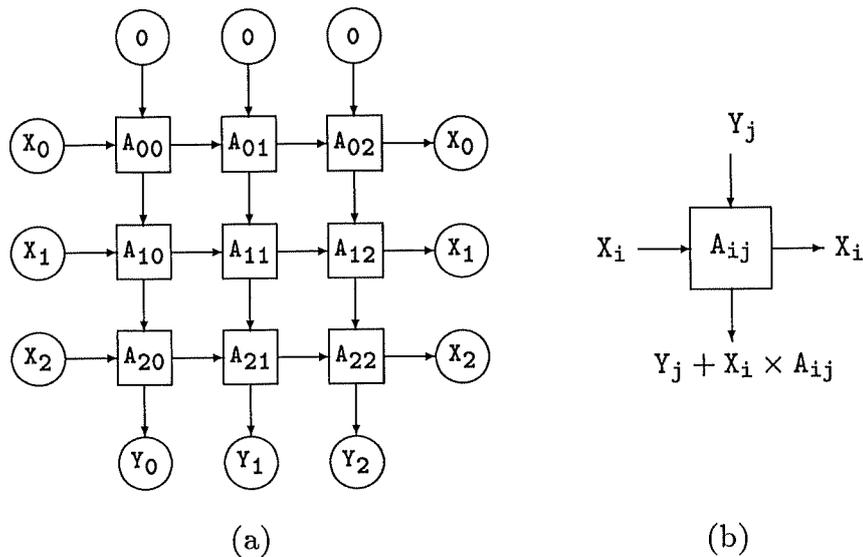
Figure 1.2: (a) A systolic array for multiplying a stream of vectors  $X$  by a constant  $3 \times 3$  matrix  $A$  giving a stream of product vectors  $Y$ ; and (b) a single cell, showing inputs and outputs.
