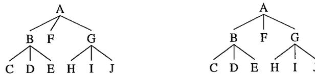
4. Identical subtrees should be rendered identically—their position in the larger tree should not affect their appearance. Again, the tree on the left fails the test, and the one on the right passes.
