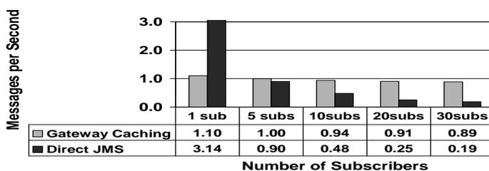
Fig. 13. Performance improvement by RemoteGateway Caching
