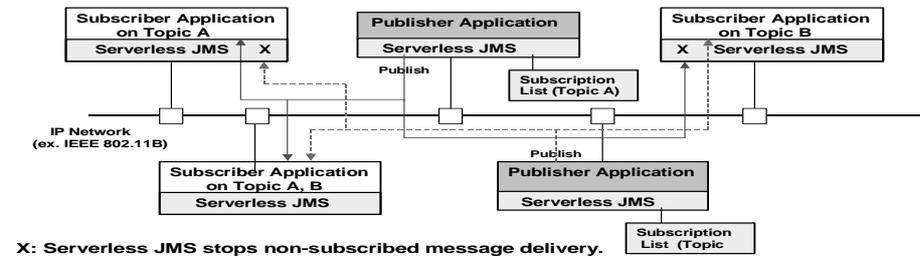
Fig. 2. Serverless JMS over IEEE 802.11 Network
