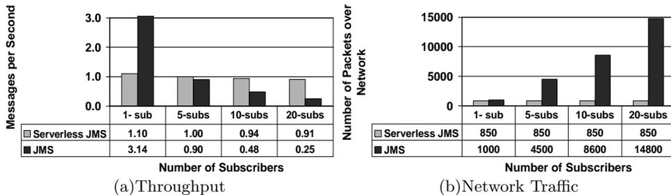
Fig. 15. Performance comparizon between JMS and Serverless JMS
