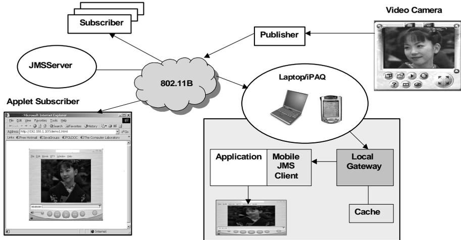
Fig. 11. Demo: Time Series of Video Data Publishing over 802.11B Network
