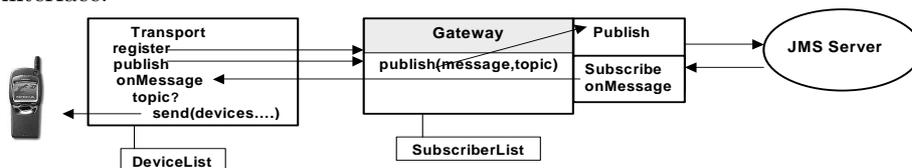
Fig. 6. Non-Programmable Devices and RemoteGateway
