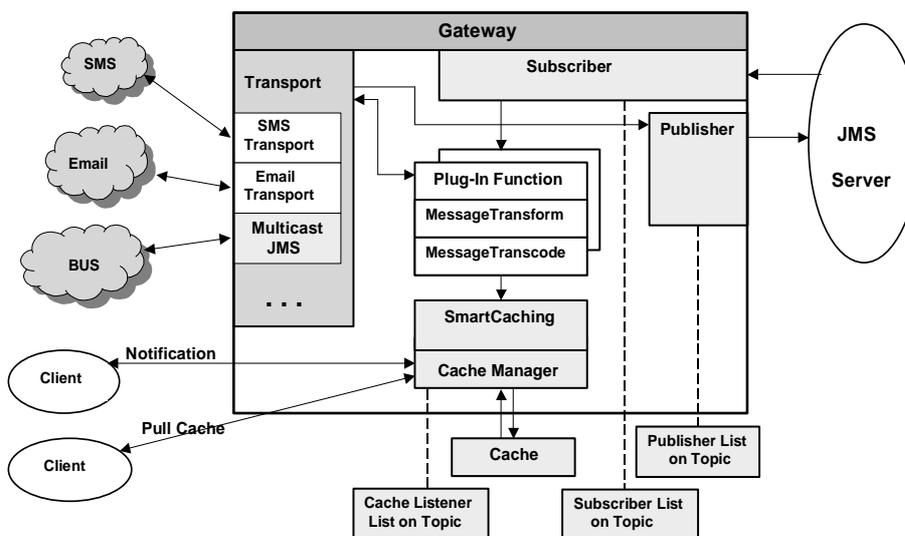
Fig. 5. Overview of Gateway Operation
