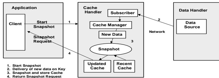
Fig. 9. SmartCaching: Snapshot Data Flow
