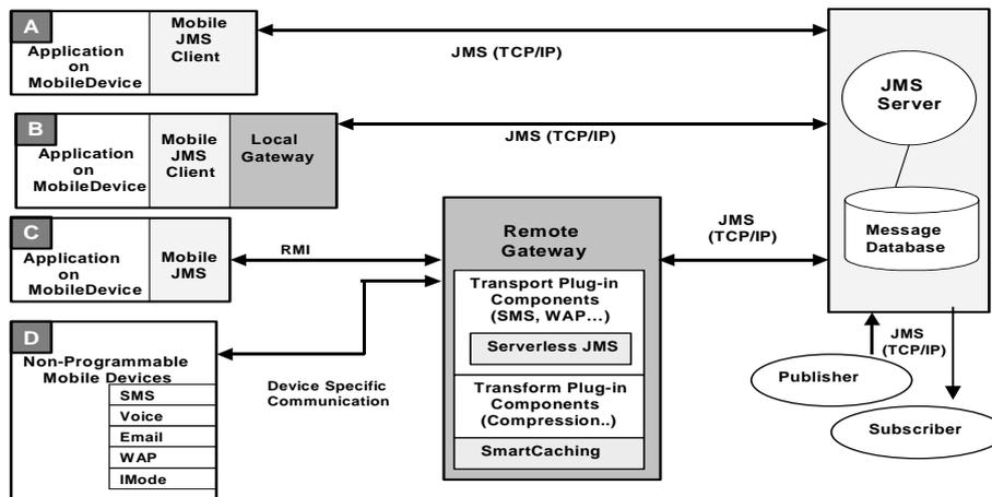
Fig. 1. System Overview of Distributed System with Pronto
