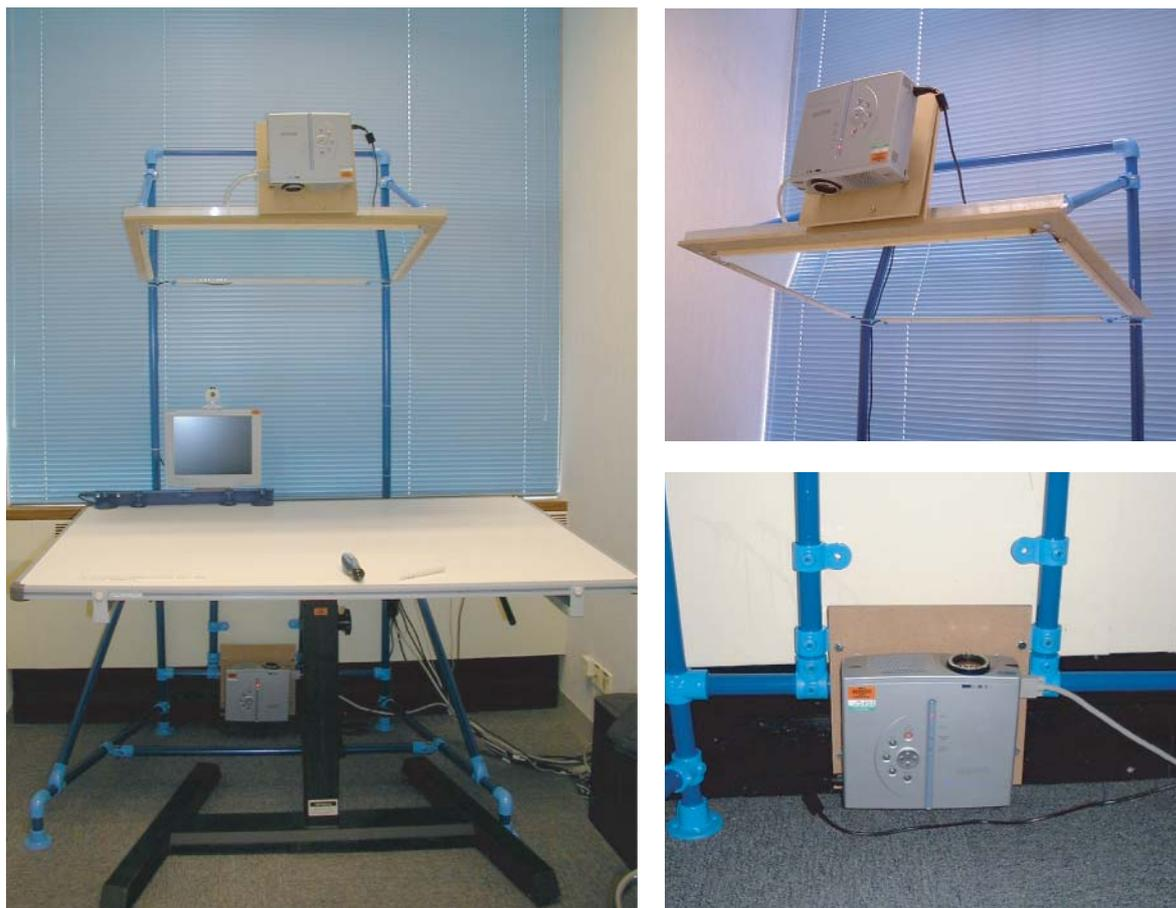
**Figure 3.8:** The second version of the Escritoire hardware. A purpose-built frame (left) holds the two projectors and the large mirror. The top projector is mounted at a steep angle (top right) so there is no need for a mirror to reflect it's image downwards. The bottom projector (bottom right) points upwards, towards the large mirror.
