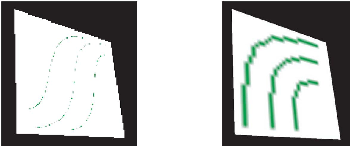
**Figure 4.9:** The scale factor from texture to framebuffer should be between 0.5 and 2.0. If the texture has too many pixels (left) some of them will be omitted. If the texture has too few pixels (right) the resolution of the projector will not be fully exploited.
