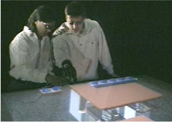
**Figure 2.23:** The Two-user Responsive Workbench [ABM<sup>+</sup>97]. Each of two users is presented with a stereo image so they can work together on the same 3D model. The users wear shutter glasses and their heads are tracked so the model can be rendered from their separate view-points.
