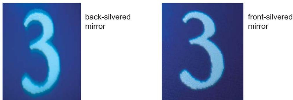
**Figure 3.9:** Difference in image quality when using front-silvered and back-silvered mirrors. The first image has been reflected onto the desk using a normal, back-silvered mirror and exhibits unwanted multiple reflections. The second has been reflected using a front-silvered mirror and does not have those multiple reflections. Each ‘3’ is approximately  $35 \times 60$  pixels and its size on the desk is about  $30 \times 50$  mm.
