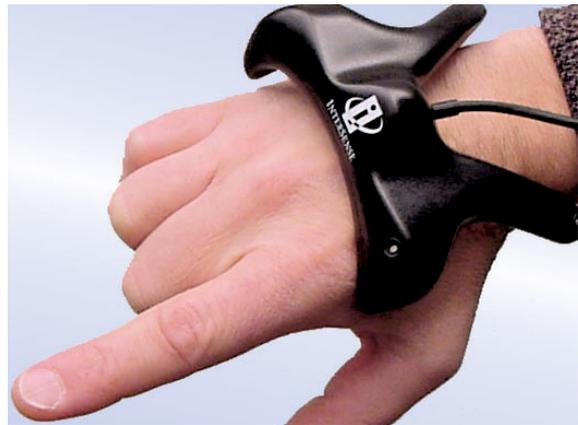
**Figure 8.1:** The Intersense MiniTrax ultrasonic hand tracker [MT]. A device like this would avoid the problems that a magnetic tracker has with metal objects, and would leave the hand free to hold a pen.
