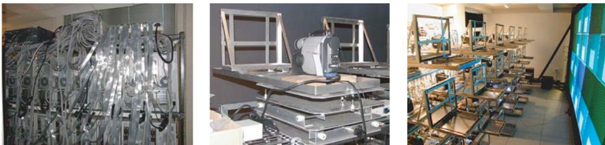
**Figure 2.11:** The Princeton display wall: (left) the cluster of PCs that drive the projectors, linked by a fast network; (centre) a projector on its mounting that has six degrees of freedom and a shadow mask to restrict the projected image to an adjustable rectangular area; (right) the array of 24 projectors.
