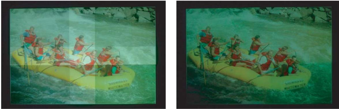
**Figure 2.14:** Photometric calibration of a multi-projector display [MS03]. Without calibration (left) the  $2 \times 2$  projector array is much brighter in the overlap regions. The images from the projectors are selectively attenuated (right) to achieve uniform brightness across the whole display.
