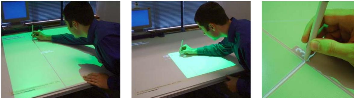
**Figure 4.5:** The user calibrates the image warping process by selecting targets projected by the (left) peripheral and (centre) foveal projectors. Each target (right) provides one point correspondence that is used in the homography calculation.
