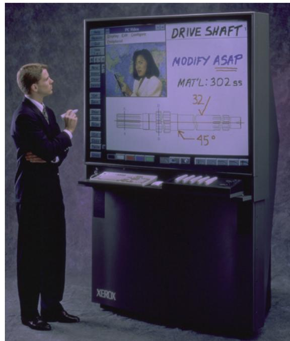
**Figure 2.4:** The Xerox Liveboard is an example of a large display device. The original was a 4×3 foot, 1120×780 pixel, rear-projected display driven by the X Window System and controlled by a laser pen tracked by a camera behind the screen [EBG<sup>+</sup>92].
