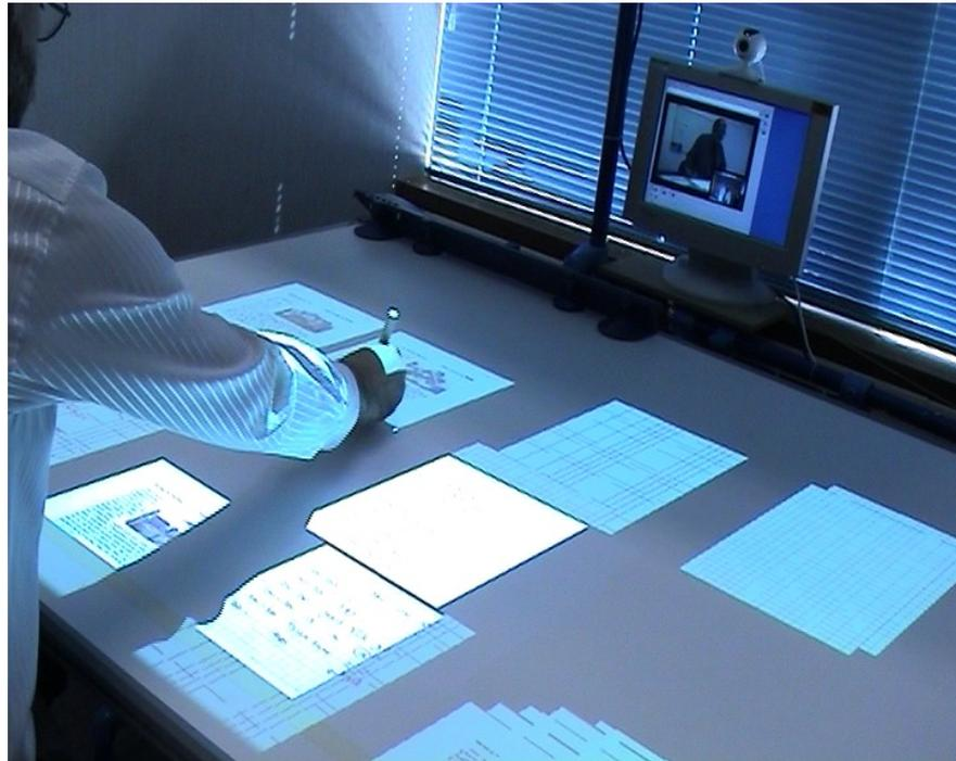
**Figure 7.10:** Sharing a task space. These two participants from the collaborative tests are in different cities, and are talking over the video link while interacting with the desk contents, which are available to both of them. The remote participant is visible on the screen in the top-right. The local participant is moving a sheet on the desk.
