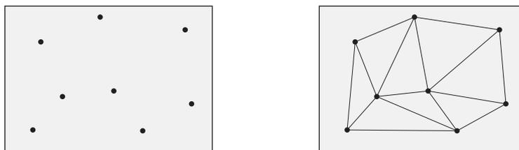
**Figure 5.3:** Delaunay triangulation: The control points (left) are joined to form a triangular mesh (right). This allows new events inside the convex hull of the control points to be assigned to an inner region, after which they are mapped using linear interpolation.
