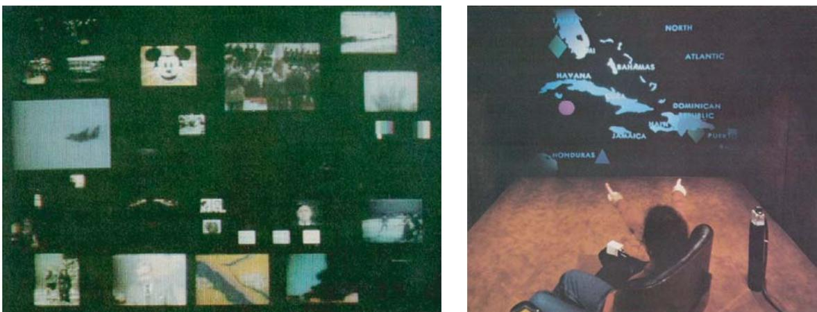
**Figure 2.7:** Early work on very large displays was done in the MIT Media Room: (left) the World of Windows [Bol81] presented the user with a wall full of video streams from which one could be selected to view in detail; and (right) Put-that-there [Bol80] used voice recognition and deictic gesturing to modify the items on the wall-sized display.
