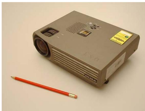
**Figure 3.1:** Projectors are getting smaller and cheaper. This is a Proxima DX3: dimensions 245×195×68 mm, weight 2.3 kg, resolution XGA (1024×768), brightness 1100 lumens, cost under 2000 euros.
