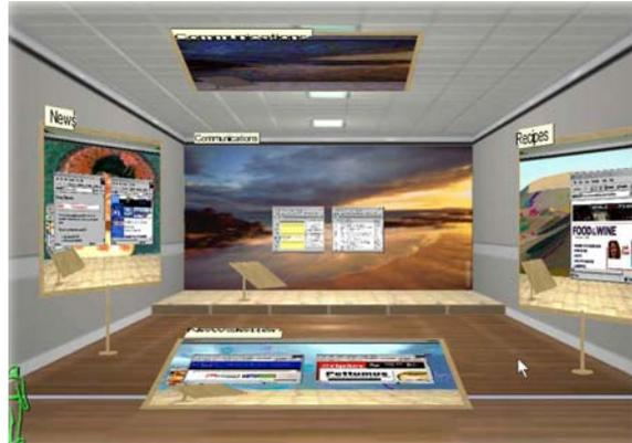
**Figure 2.1:** Microsoft’s Task Gallery [RvDR<sup>+</sup>00] allows more tasks than usual to be managed on a conventional monitor by representing virtual workspaces as paintings in a 3D gallery metaphor.
