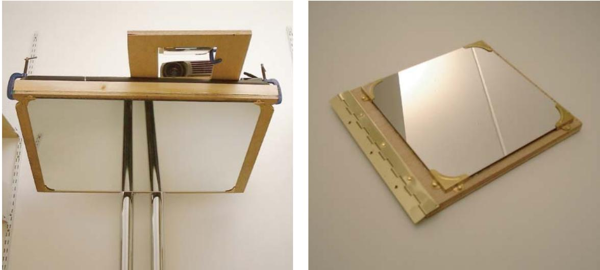
**Figure 3.7:** In the first version of the Escritoire hardware the projector for the fovea (left) was placed on top of the shelf above the desk that holds the large mirror, and had a smaller mirror (right) that reflected it's image down onto the desk surface.
