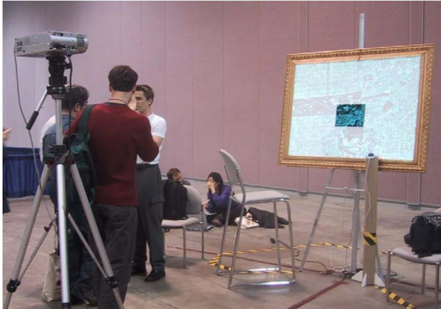
**Figure 2.9:** The focus plus context screen [BGS01] is a standard front-projected display with an LCD monitor set into the screen to create a high-resolution focal area.
