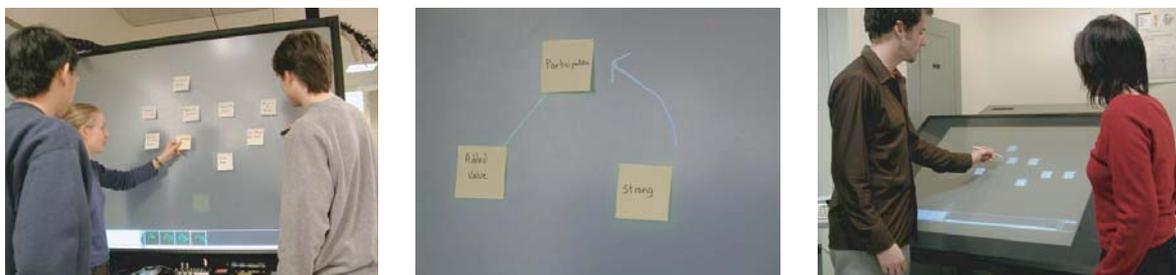
**Figure 2.29:** The Designer's Outpost system [EKLL03] is designed to allow participants in different locations to work with the same arrangement of paper notes. Those at one end can manipulate the physical notes. A remote user can move a note's virtual counterpart which then indicates an inconsistency that the local user must correct by moving the physical note to its new position.
