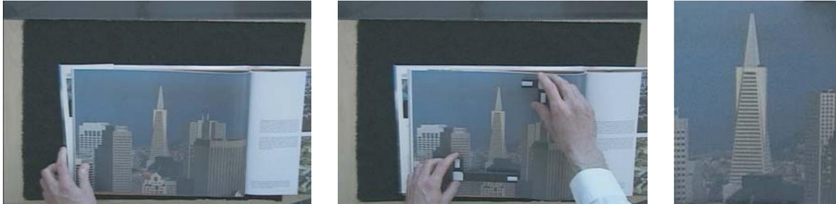
**Figure 2.20:** FlowScan [Gui02] allows pictures to be added to the Stanford Interactive Mural. The user puts a picture in position (left), places crop markers on it (centre), then a camera automatically samples the picture (right) and places a copy on the display wall.
