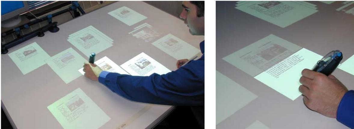
**Figure 6.5:** PDF Portfolios: (left) many sheets of PDF are arranged on the desk surface; (right) the user can bring any sheet to the fovea to view it in detail.
