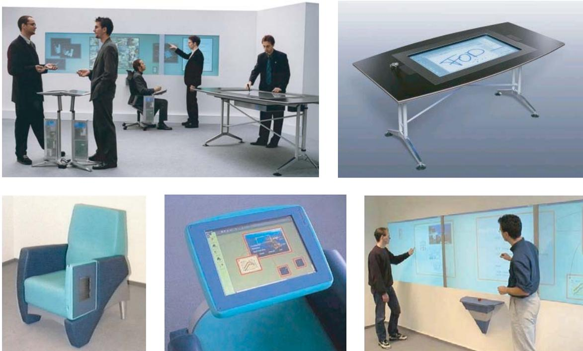
**Figure 2.26:** Roomware [PT02] components allow collaboration around displays of different types with varied affordances (top left). The *InteracTable* (top right) allows many users to gather around, the *CommChair* (bottom left and bottom centre) provides a private workspace, and the *DynaWall* (bottom right) presents a large workspace on which users can work separately or collaboratively
