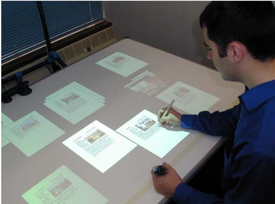
**Figure 1.7:** The *Escritoire*. It has a horizontal display the size of a desk that accepts input from a pen in each of the user's hands. One projector fills the desk, and a second creates a high-resolution area in front of the user for detailed work. Several desks can be linked via a network to allow collaboration in which the sheets of virtual paper can be manipulated by all participants.
