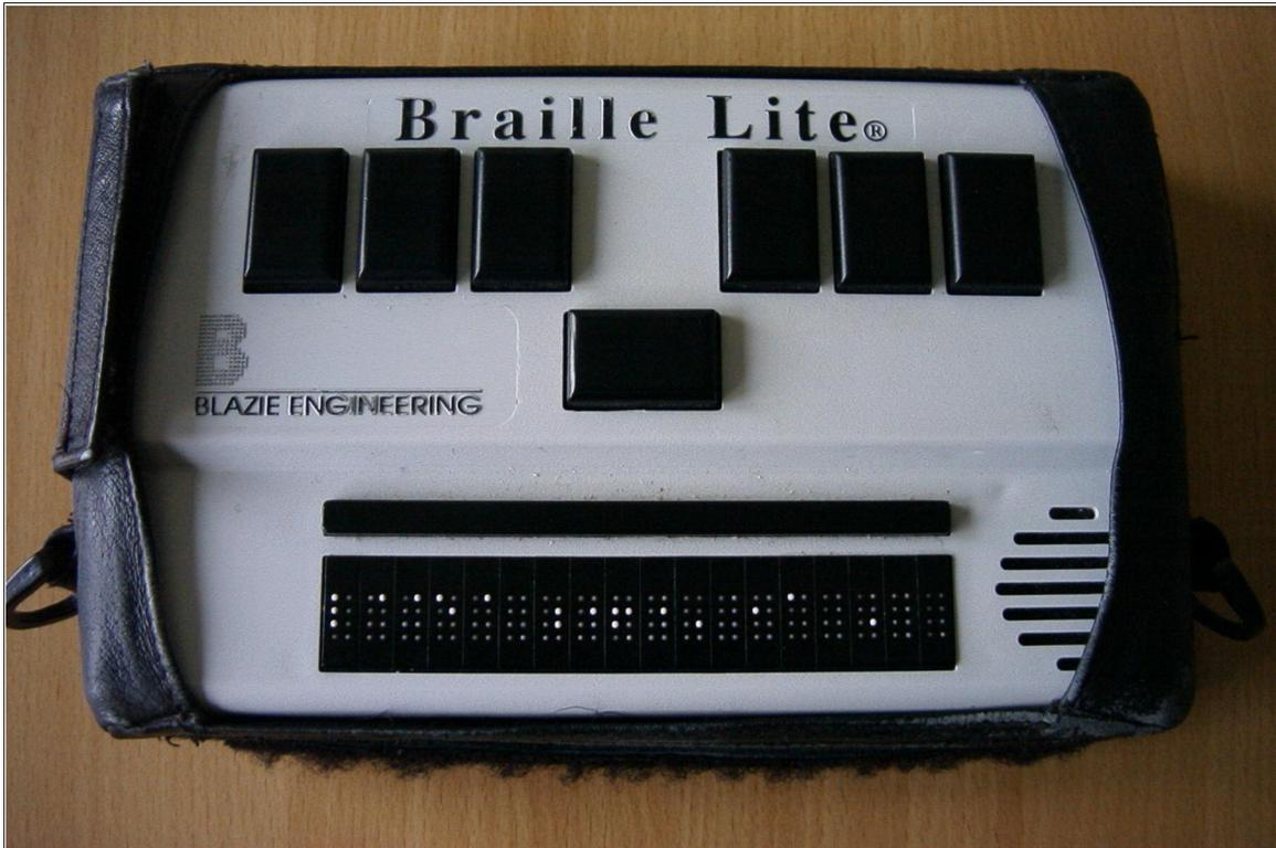
Figure 5.30: Braille-based note-taking device (photo: Hans Schou)
