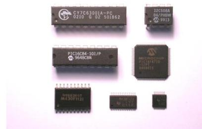
Figure 16. Microcontrollers with OTP EPROM, EEPROM and Flash EEPROM
