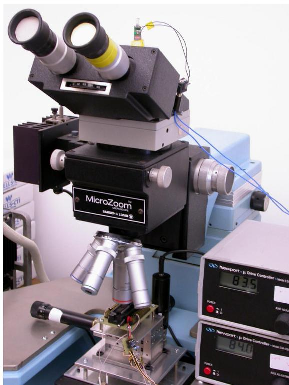
Figure 80. Laser scanning setup with the laser pointer on top of the microscope and a moving sample under it
