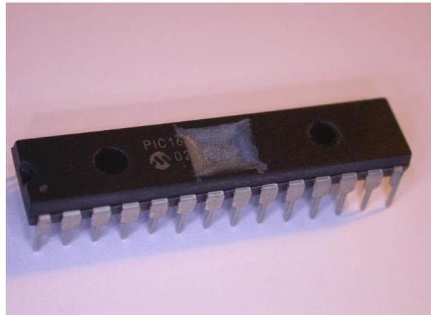
Figure 50. Mechanical grinding tool for plastic packages preparation for manual decapsulation and pre-milled chip in the DIP package
