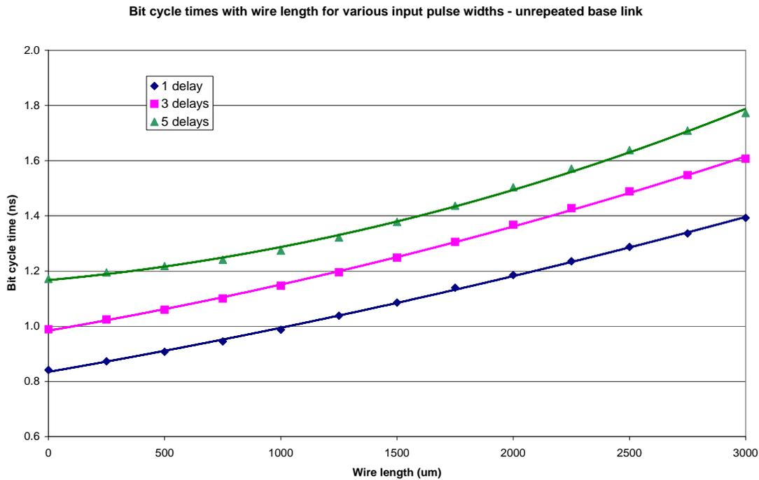
**Figure 6.35:** The effect of interconnect length on bit cycle times — pulse chopper unrepeated base link
