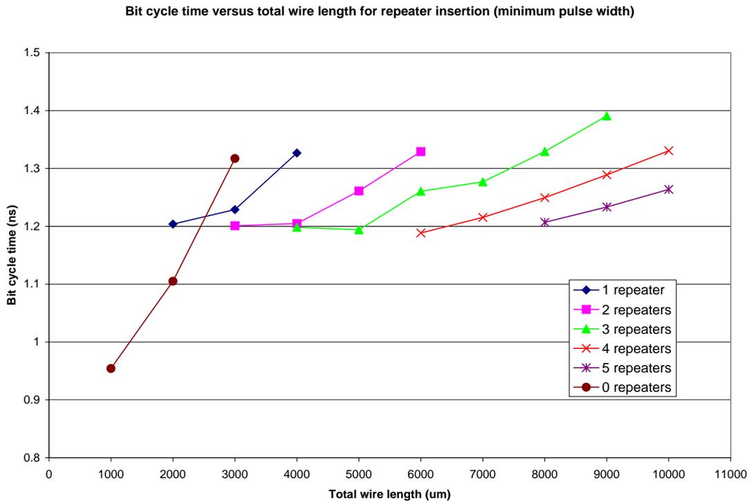
**Figure 6.29:** Bit cycles times for a MUX-DEMUX link with total wire length, for varying numbers of repeaters inserted — flop pulse generator, 1 delay
