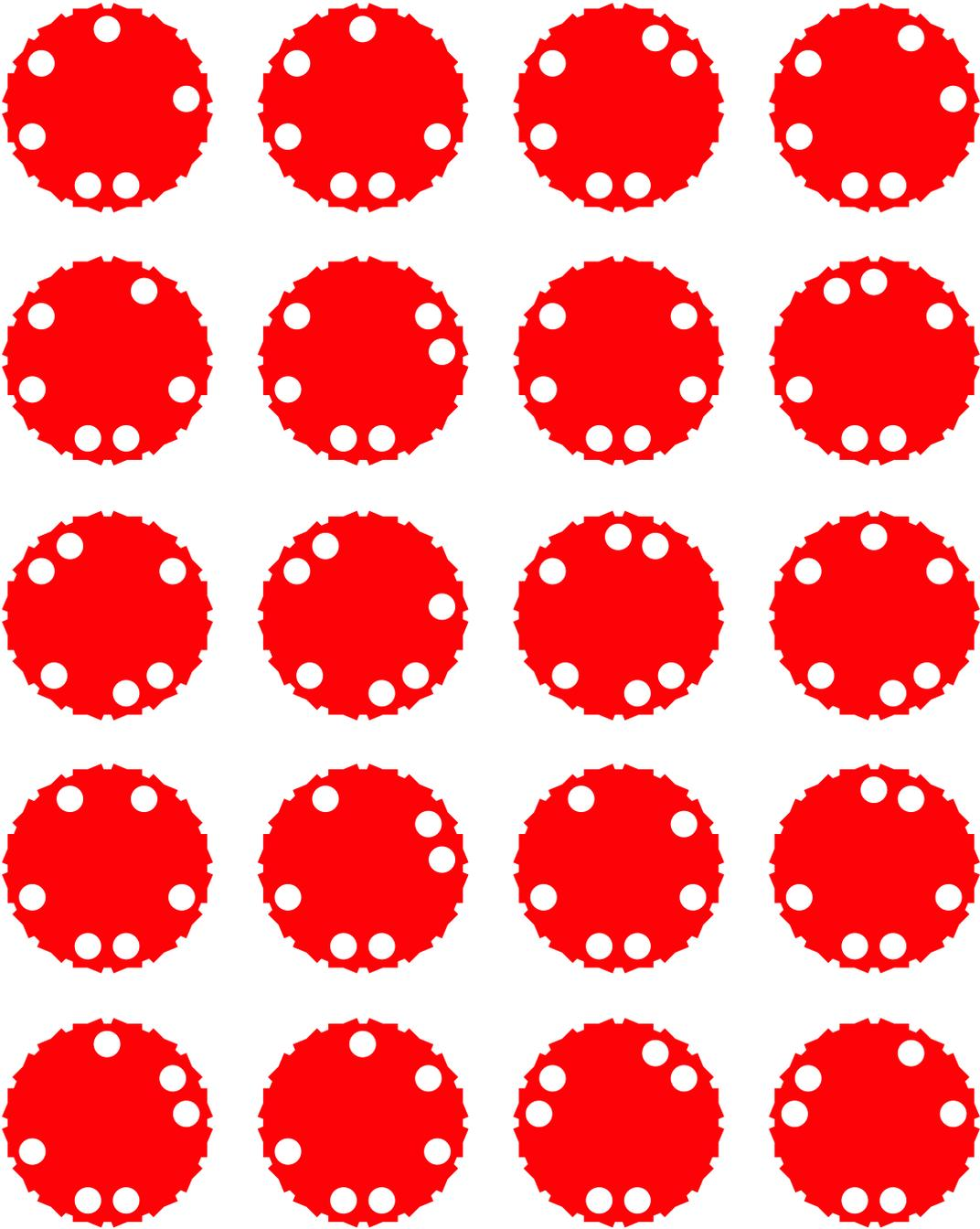
Figure A.5: Sample of Vector Graphics Token Specifications: A set of 20 matching task tokens belonging to a single user, created in Adobe Illustrator based on the output of my "token sheet generator" written in Java. Tokens were laser-cut directly from these specifications.
