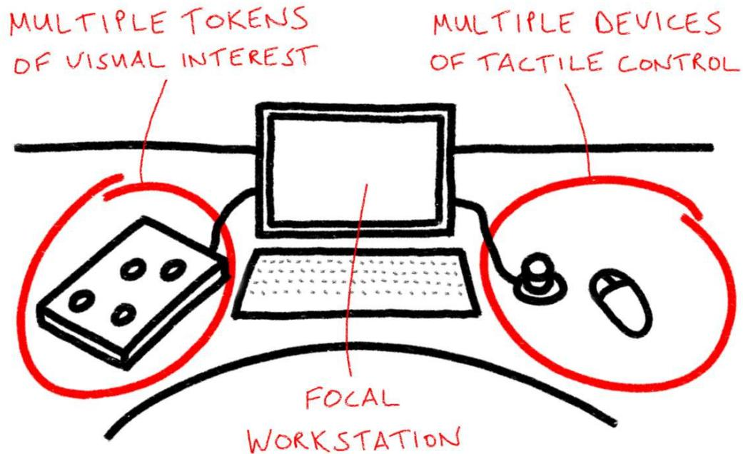
Figure 4.4: Design Sketch of a Bimanual TUI for Peripheral Interaction
