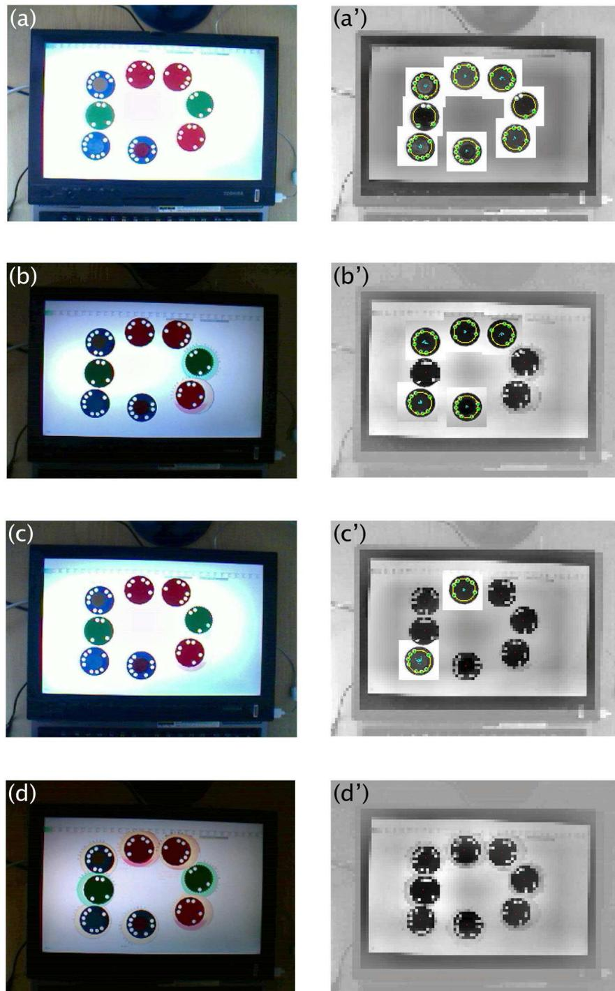
Figure A.8: Token Tracking Using State Machines and Position Matching: (a-d) as the cover is removed from the Webcam, it automatically recalibrates; (a') all 8 untracked tokens are decoded; (b') 3 tokens have repeatedly given the same code so can be tracked frame-to-frame based on their position; (c') 2 tokens remaining untracked; (d') all tokens tracked based on their low-resolution position.
