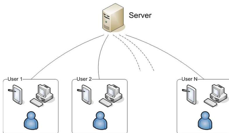
Figure 5.5: Client-Server Architecture, Multiple User View: Multiple pairings of workstation and interactive surface communicate with a single server.
