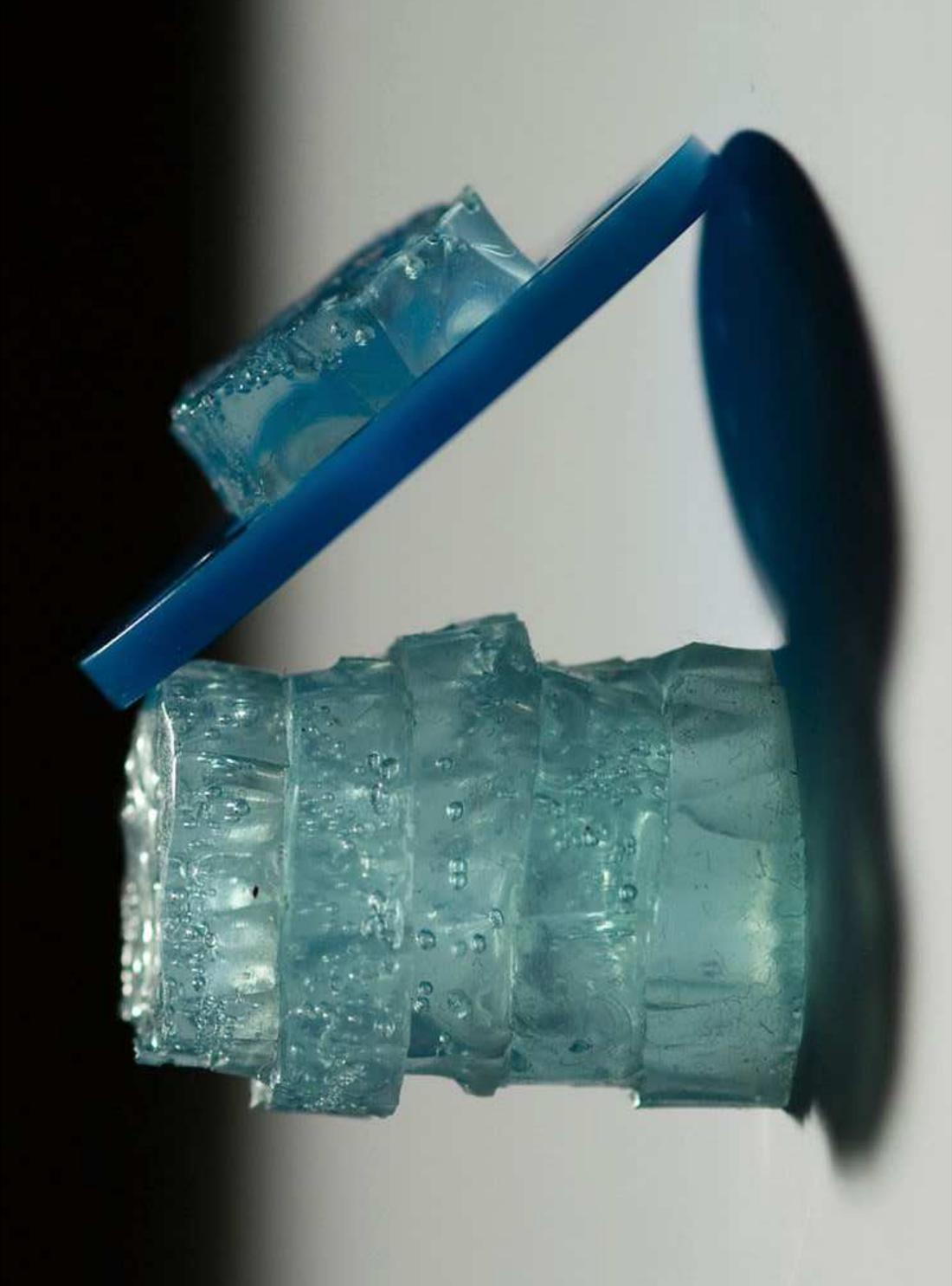
Figure 5.19: Example Attachment Material for Document Tokens: Silicone Gel
