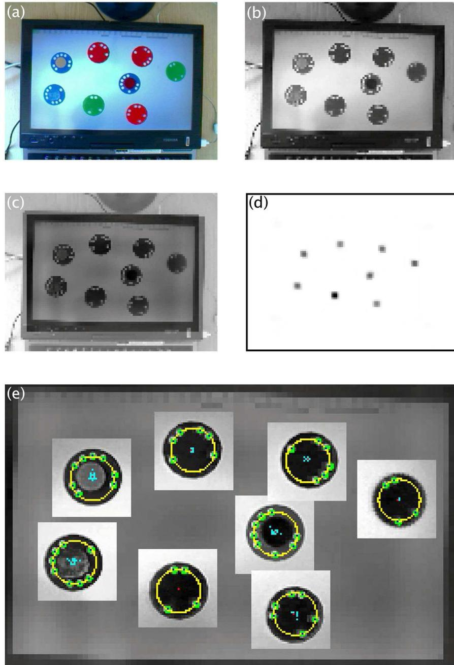
Figure A.7: Token Detection and Identification (2): (a) the high-resolution, colour Webcam image; (b) a low-resolution simple greyscale image (not used); (c) a low-resolution greyscale image based on a weighted combination of saturation and smoothed brightness; (d) response of a fast radial-symmetry 'token' detector; (e) high-resolution 'windows' around potential tokens examined for token holes. Note the harsher brightness gradient across the tablet screen compared with Figure A.6.
