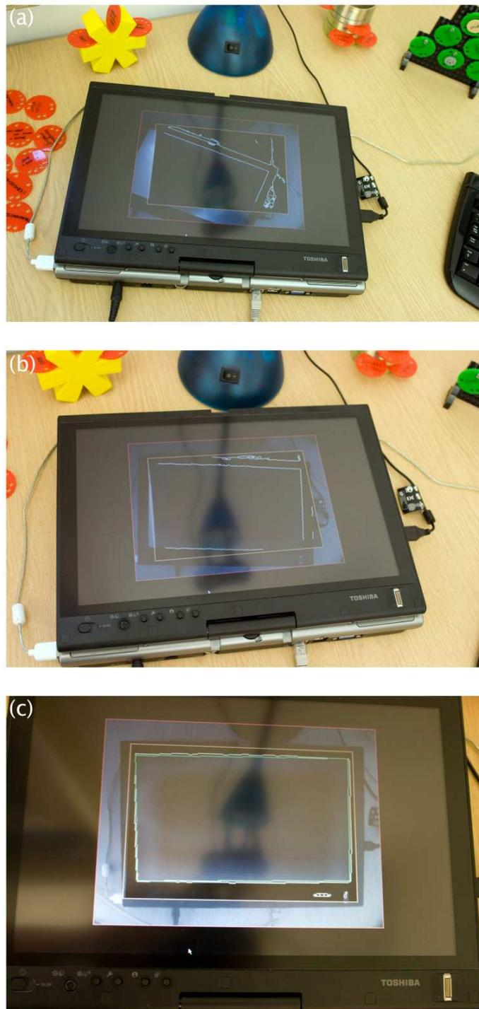
Figure A.4: Interactive Camera-Surface Calibration: (a,b) feedback as to the relative positioning of the Webcam and tablet PC guide the user to slide the tablet PC into the correct alignment; (c) all four corners of the tablet PC are within the target region – the user may proceed to system usage.
