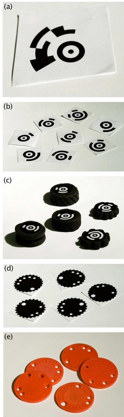
Figure 5.9: Evolution of Token Prototypes: (a) an original TRIP code; (b) my modified TRIP codes – compact, single-ringed circular codes; (c) "3D sketches" using plasticine; (d) paper mock-ups of token codes based on patterns of holes; (e) pre-production plastic prototypes constructed by drilling holes in poker chips.
