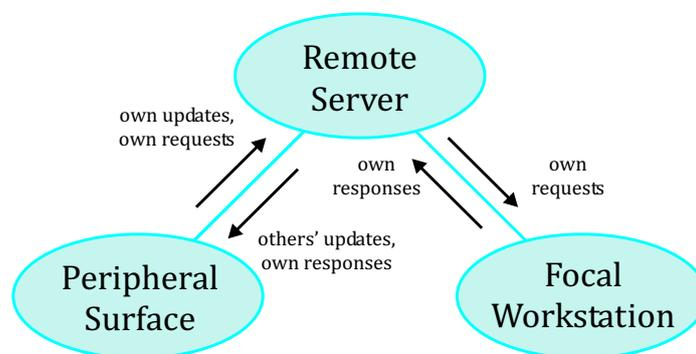
Figure 5.6: Client-Server Architecture, Single User View: The peripheral surface sends requests for user input to the focal workstation, which relays responses back to the interactive surface.
