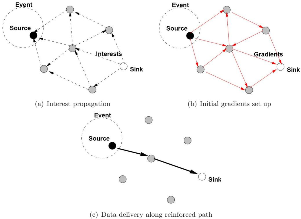
Figure 2.2: Schematic diagram for Directed Diffusion
