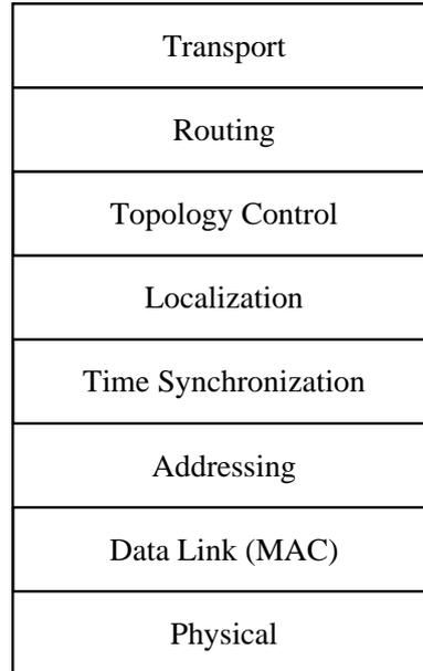
Figure 2.1: Communications protocol stack
