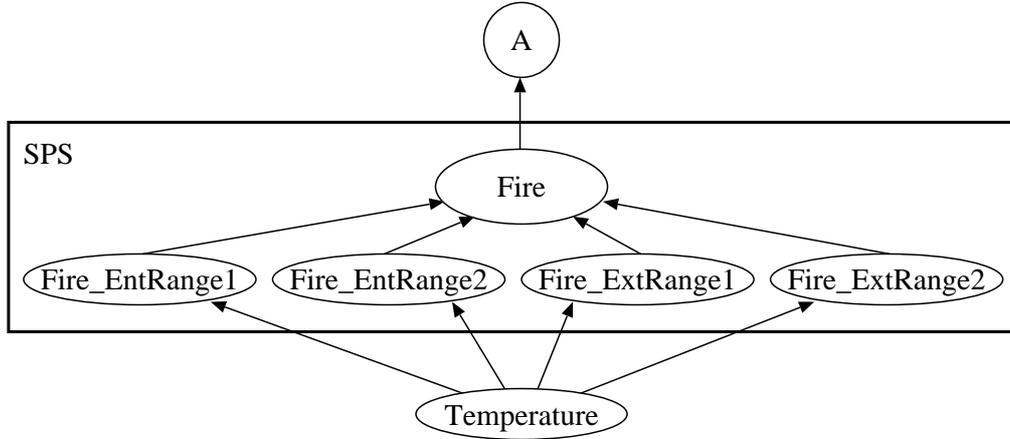
Figure 5.12: Decomposed fire detection information flow
