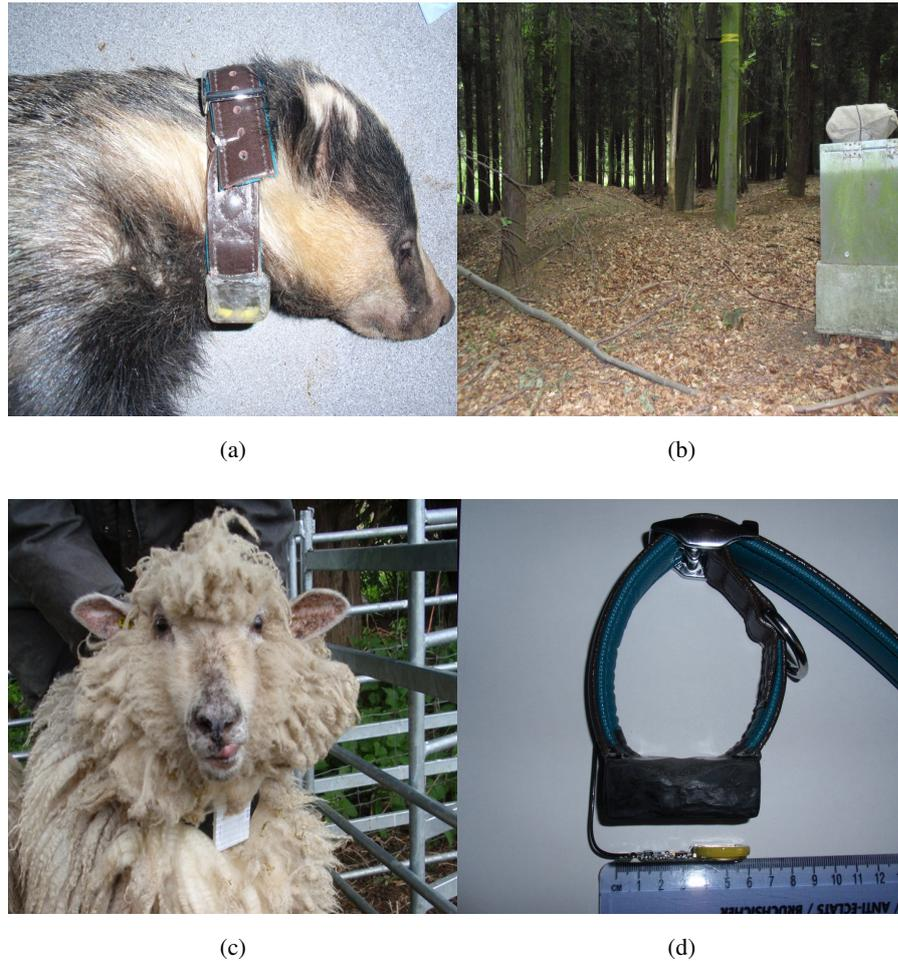
Figure 7.2: RFID system deployment. a) a tagged badger carrying a potted RFID tag. b) RFID node deployed near the badger burrow. c) RFID tagged sheep during early field tests. d) OEM-TM100 RFID active tag and a collar.
