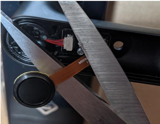
(c) Attacking the sensor with scissors
