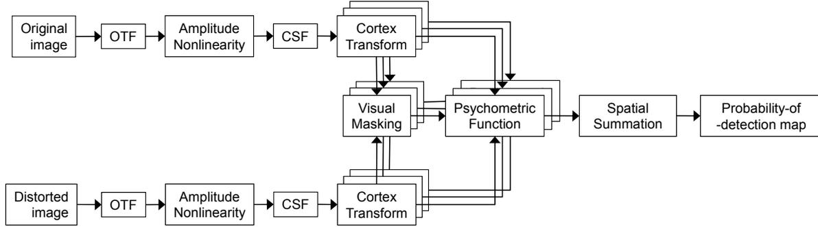
Figure 2. The block diagram of the HDR-VDP.
