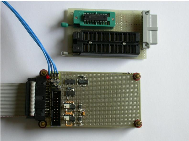
**Fig. 1.** The test board for data remanence evaluation
