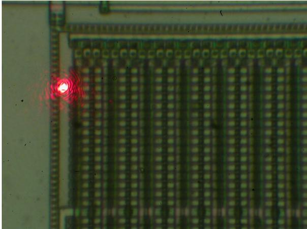
**Fig. 3.** Focusing the laser with a 100× objective
