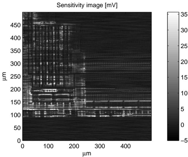
**Fig. 9.** Laser-scanned image of the ATmega8 EEPROM area
